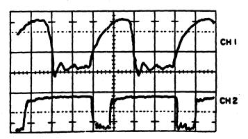
NOTE: SET DISPLAY MODE TO ALT AND TRIGGER MODE TO CH 1 ONLY. Also set horizontal display to b (delayed sweep)
