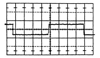
RM05 Data Latch Output Waveform
